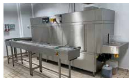
Molds washing tunnel
