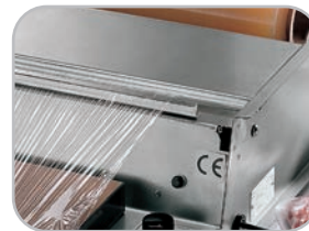
Particolare filo caldo (1) Heated cutting tread (1)
